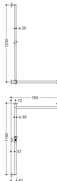
Abmessungen in mm
