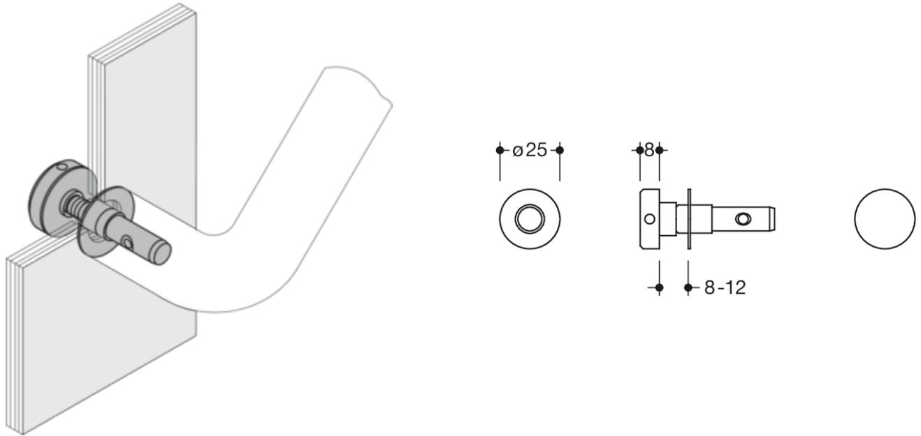
Abmessungen in mm
