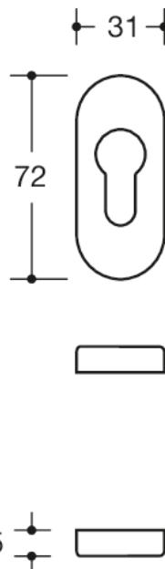
Abmessungen in mm
