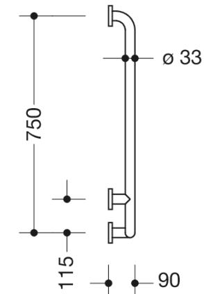
Abmessungen in mm
