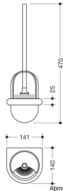
Abmessungen in mm
