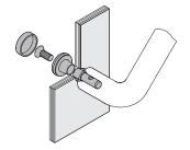
BA4.08.12\* BA4.08.12B\* HEWI Fixing type 4.08.12 for pull handles made of polyamide HEWI Fixing type 4.08.12 for pull handles made of matt polyamide
