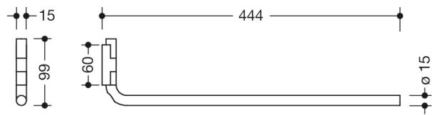
Technical drawing showing dimensions for the towel holder: height 99 mm, width 60 mm, depth 15 mm, and overall length 444 mm. The support arm has a diameter of 15 mm.
