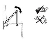
Check friction on both sides of the seat.
