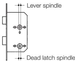
Lever spindles available: 8, 8,5, 9 and reduced 10 to 8 mm..
