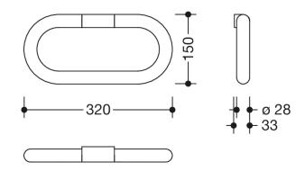
Abmessungen in mm
