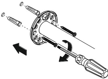
Use extended bit acceptances (approx. 4 in) when using electric screwdrivers or similar as otherwise the chuck may damage the surface!
